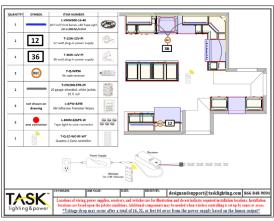
Sample layout from Design Services showing LED tape lighting
